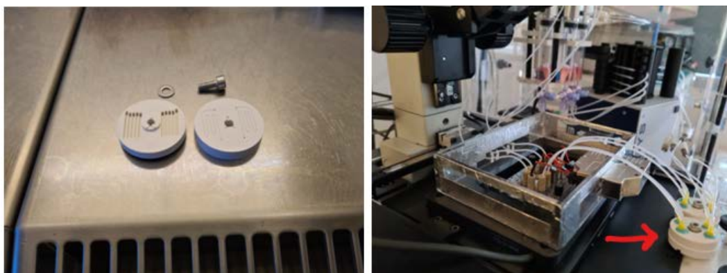
Fig. 26. Bubble traps (Left) and bubble traps connected to the microfluidic system (Right).
